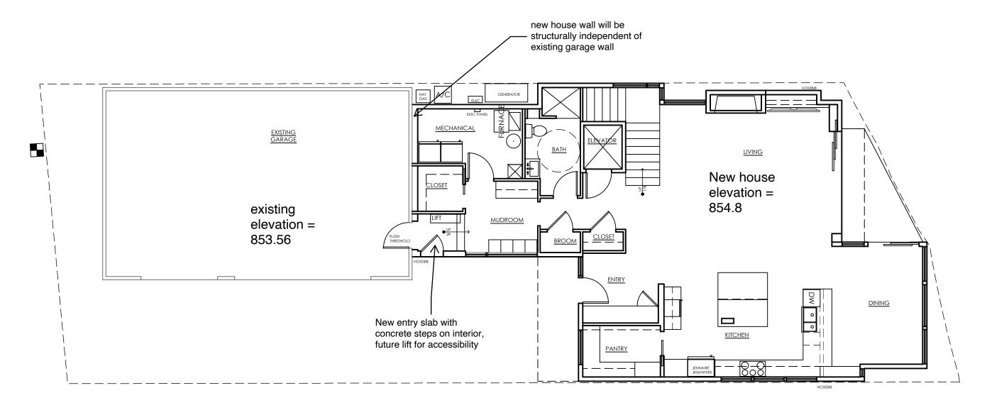
Note: New house - construction to be Concrete Insulated Form foundations with insulated slab at new grade createing a finished floor elevation of 854.8.
