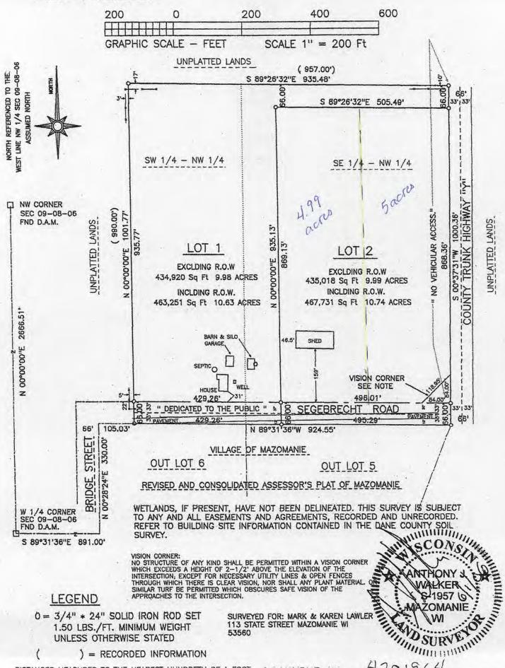
DISTANCES MEASURED TO THE NEAREST HUNDRETH OF A FOOT BEARINGS MEASURED TO THE NEAREST 5"
