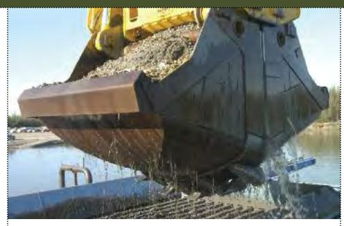
This photo shows sand and gravel extraction below the water table. Gravel is removed, leaving the water table intact.
