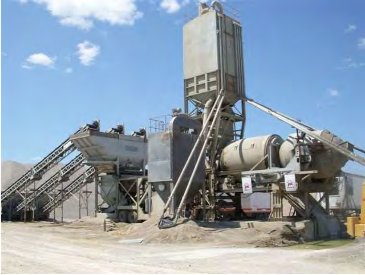
FIGURE 3 – MICHELS CONCRETE BATCH PLANT
