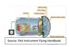
While altitude accuracy is desired, barometric altimeters have inherent errors. The acceptable error for an altimeter is 75 feet, according to FAA guidance.
