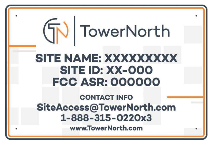
TOWERNORTH SIGN WHITE/ BLACK BACKGROUND, BLUE LETTERING. MOUNTING LOCATION: GATE QUANTITY: 1 WHERE ACCESS GATE INSTALLED AND COMPOUND IS NOT VISIBLE FROM MAIN ROAD (QTY. 2) (PROVIDED BY TOWER OWNER)
