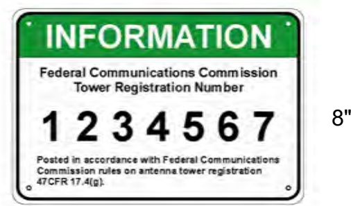
FCC REGISTRATION SIGN WHITE/ GREEN BACKGROUND, WHITE/ BLACK LETTERING. MOUNTING LOCATION: GATE & BASE OF TOWER QUANTITY: 2 WHERE ACCESS GATE INSTALLED (QTY. 3)
