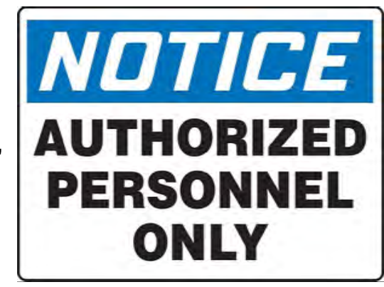
AUTHORIZED PERSONNEL SIGN WHITE/ BLACK BACKGROUND, WHITE/BLACK LETTERING. MOUNTING LOCATION: GATE & BASE OF TOWER QUANTITY: 2 WHERE ACCESS GATE INSTALLED (QTY. 3)
