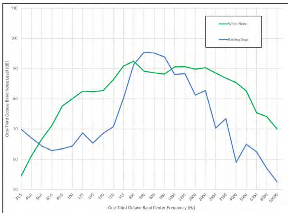
Figure 1. 1/3 Octave Band Noise Levels Produced Inside Facility
