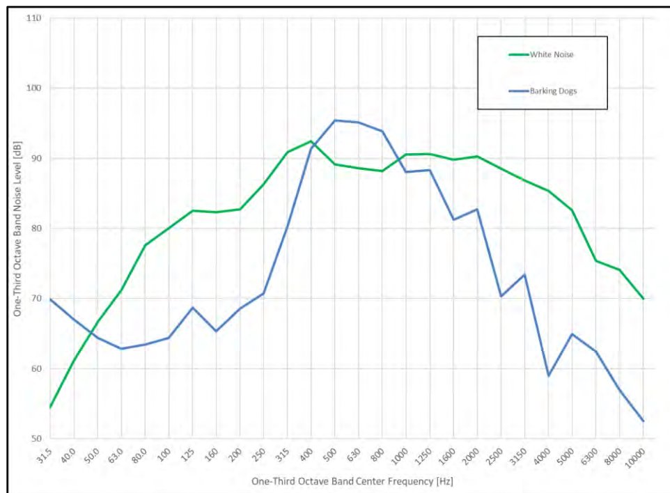
Figure 1. 1/3 Octave Band Noise Levels Produced Inside Facility
