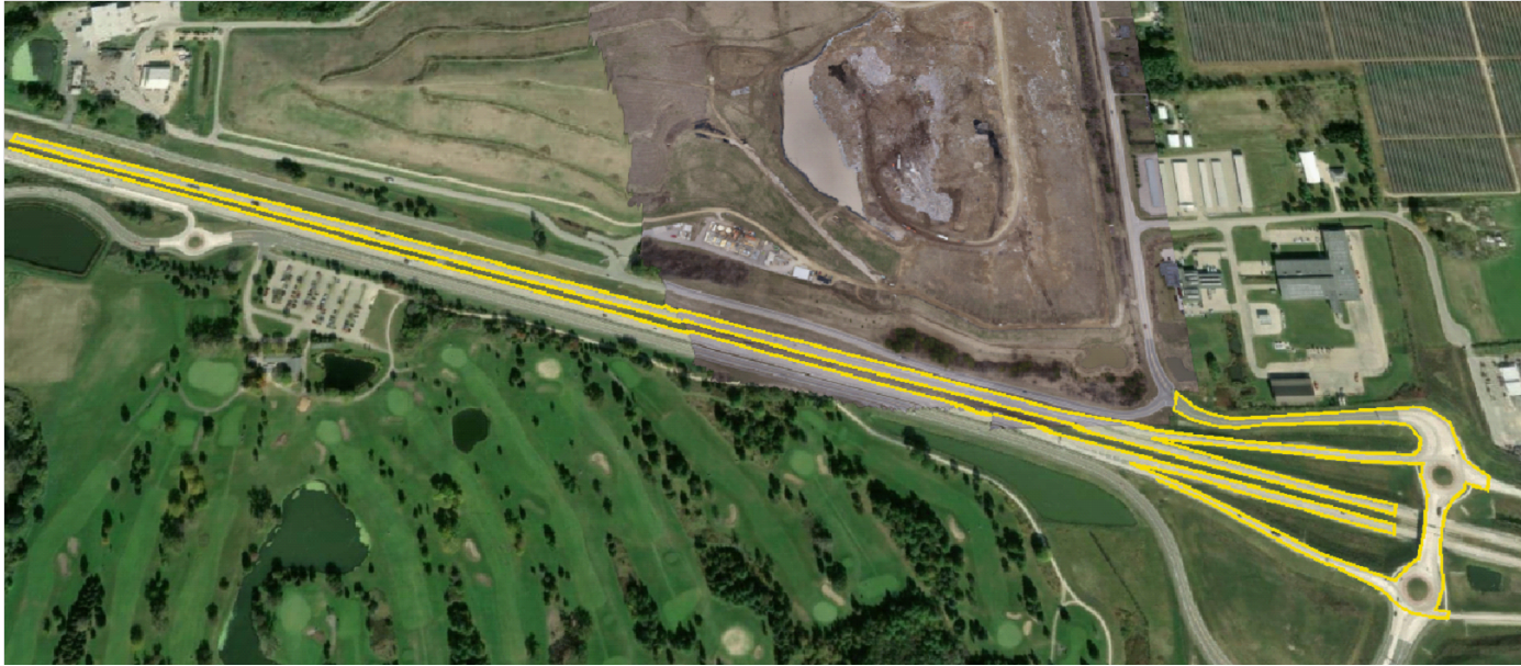
Figure A: HWY 12 & 18 (yellow line) - Includes east bound median + west bound median + west bound shoulder, through both sides of the roundabouts to both sides of the intersection of AB & Maahic Way - estimated ~27,500 LF or ~5 miles
