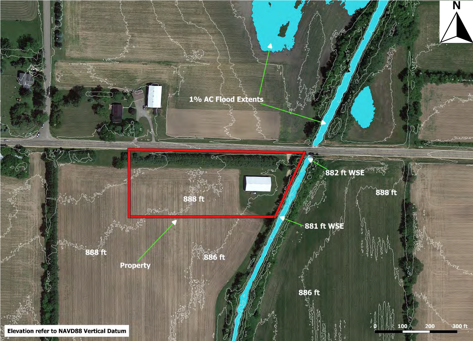
Figure 5. Maximum 1% AC flood WSE (ft) near property boundary along with 2-foot contour intervals extracted from 2017 LiDAR.
