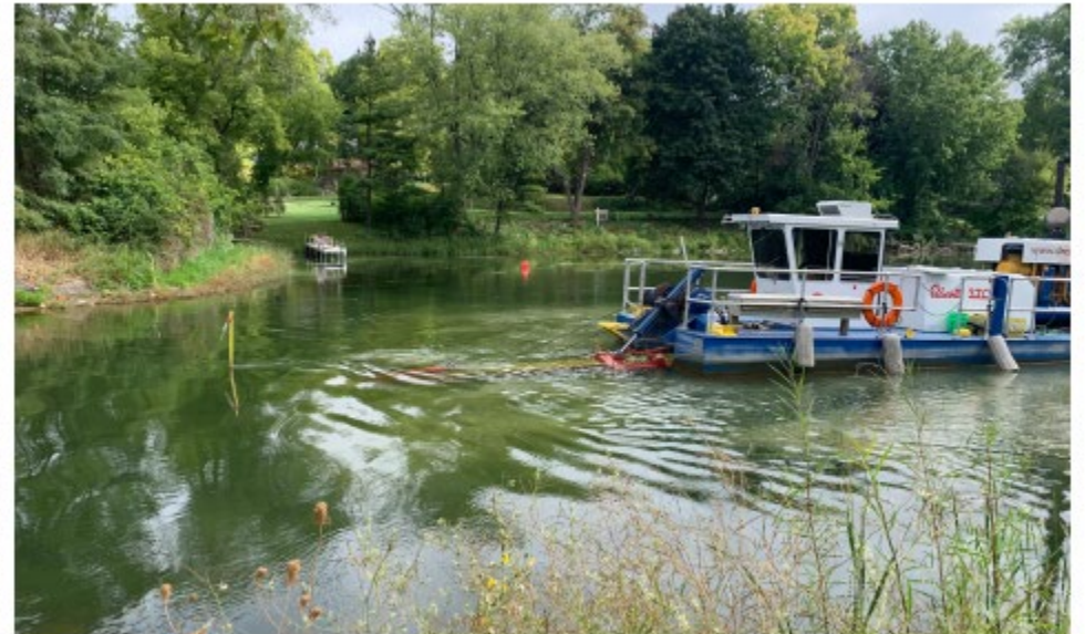
Dredge equipment removes sediment and obstructions from the riverbed.
