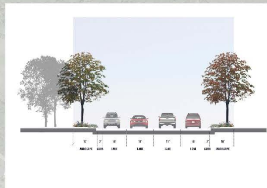
PRIMARY CIRCULATION "RING" ROAD: TYPICAL SECTION
