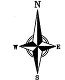
BEARINGS ARE REFERENCED TO THE WISCONSIN COUNTY COORDINATE SYSTEM, DANE COUNTY, WISCONSIN. THE NORTH LINE OF THE NW 1/4 OF SECTION 30-08-10 MEASURED AS BEARING S87°59'37"E
