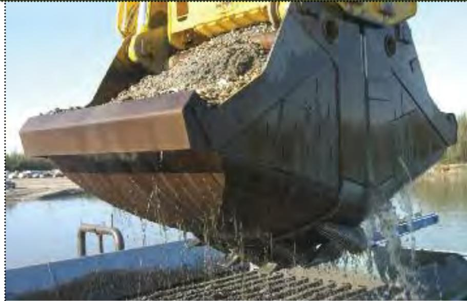
*This photo shows sand and gravel extraction below the water table. Gravel is removed, leaving the water table intact.*
