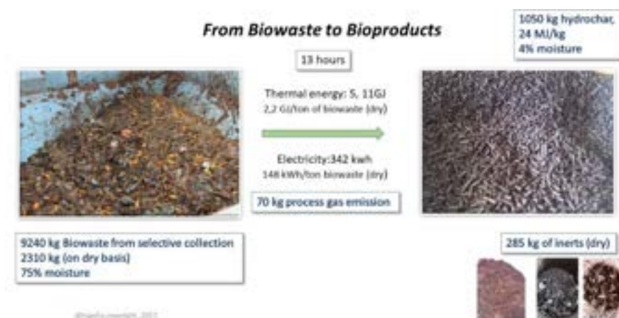
Figure 2. From biowaste to hydrochar - Example of a trial
