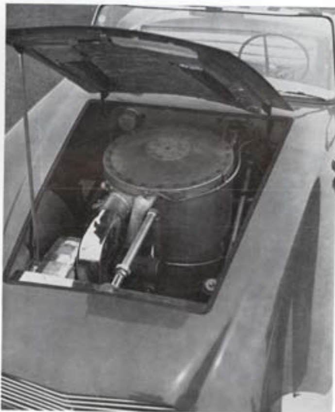
The steam generator.
