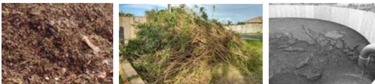
Figure 1. Waste feedstocks used in the Ingelia HTC process. From left to right: compost out of specification (30% wt. moisture); green waste (50% wt. moisture) and digestate (85% wt. moisture).
