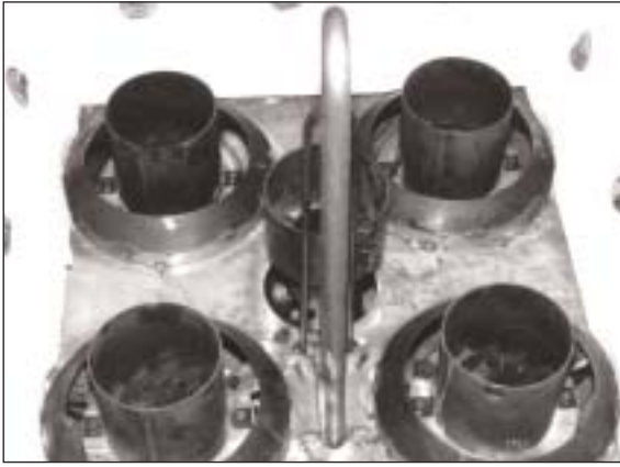
Fig. 4: Oil firing system after the tests.
