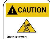
On this tower: Radio frequency (RF) fields near some antennas *may exceed* the FCC Occupational Exposure Limits. Personnel should be trained and use a personal RF monitor when working.
