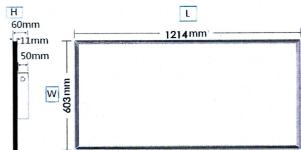
Driver Box=50x100x320mm Panel: L=1214mm W=604mm H=60mm Driver Box=1.96"x3.94"x12.6" Panel: L=47.8" W=23.8" H=2.36"
