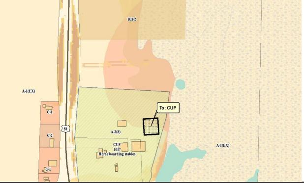
**DESCRIPTION**: The applicant, SBA Towers V / Verizon Wireless, proposes to construct a 130' tall monopole communication tower (138' total height with lighting rod) on the existing A-2(8) Agriculture zoned property located at 2660 US Highway 51 in section 10 of the town of Dunn. The tower would be engineered to be extendable up to 160' in the event a future collocating carrier required additional height for their network service needs (169' with lighting rod).
