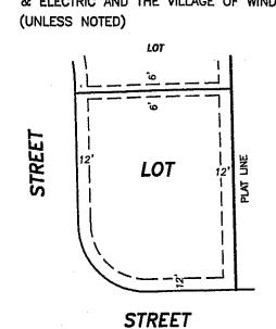
NOTE: EXISTING 12' UTILITY AND STORM WATER EASEMENTS ALONG EXISTING RIGHTS-OF-WAY PER REVERE TRAILS.
