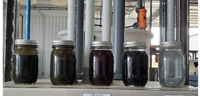
Samples of processed manure through NCS. Raw manure is on the left. Clean water is on the right.
