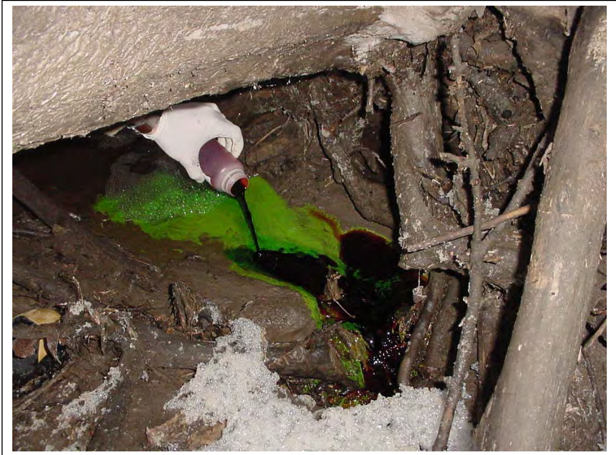
Figure 5. Introducing dye into the stream of water.
