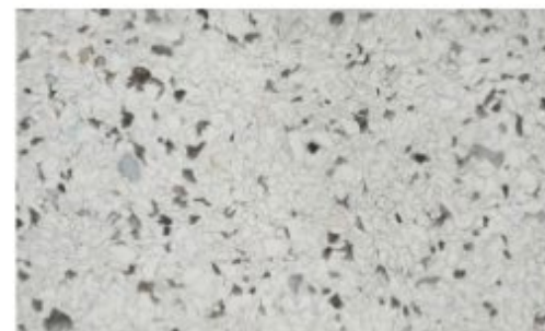
RECYCLED MATERIAL COUNTERTOP PLASTIC SOURCED FROM REFRIGERATORS/CONSUMER ELECTRONICS
