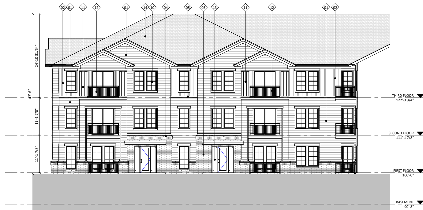
2 ELEVATION - HIDDEN NORTH A-2.3 1/8" = 1'-0"
