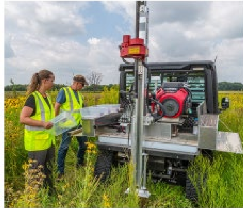
Collecting soil samples using a hydraulic coring machine mounted to the bed of a utility train vehicle.
