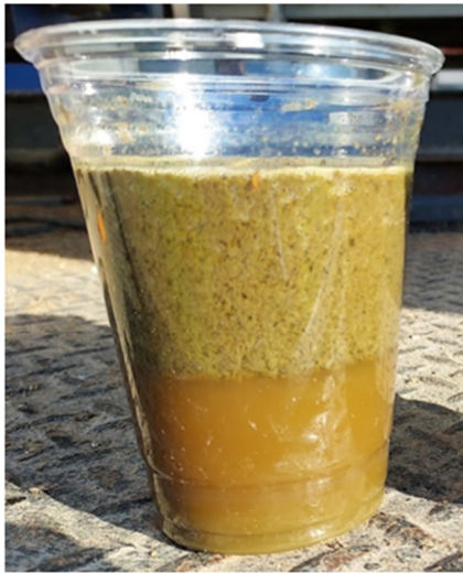
Flocculated solids (floating) and clarified liquid from dairy digestate
