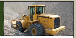
In an aggregate operation, equipment such as bulldozers, loaders, crushers and dump trucks creates noise. The intensity of sound is measured in units called decibels. Research and sound-muffling strategies help minimize noise that comes from a pit or quarry. This benefits both employees and neighbors.
